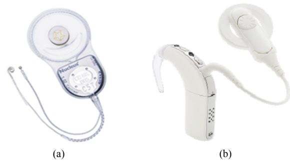
Figure 1. Cochlear implant system: (a) Internal component (Nucleus CI24RE (CA)) and (b) External component (Nucleus CP810). Photos courtesy of Cochlear™.
